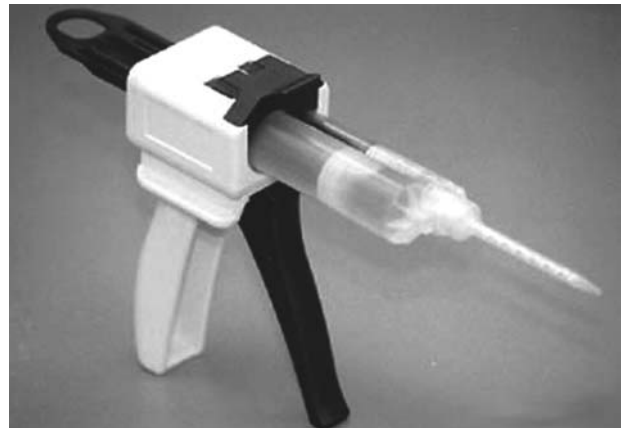
FIGURE 1-7. Applicator gun used to apply albumin cross-linked with glutaraldehyde to vascular tissues.
